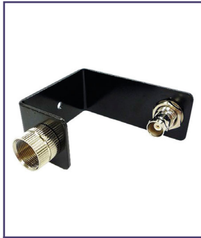
UHF410-Hold Antenna support with BNC connector
